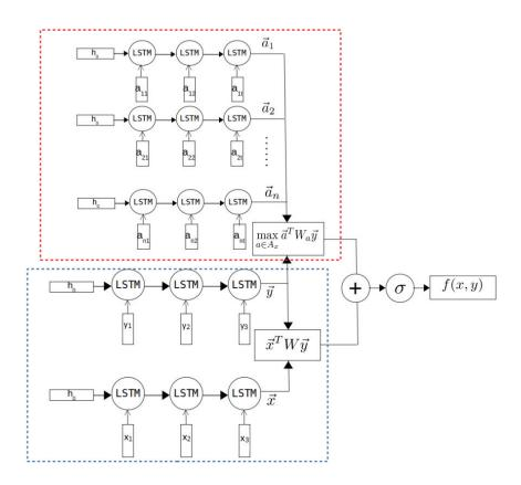
Figure 3: Tri-LSTM encoder. We use LSTM to encode message, response and commonsense assertions. LSTM weights for message and response are tied. The lower box is equal to a Dual-LSTM encoder. The upper box is the memory module encoding all commonsense assertions.
